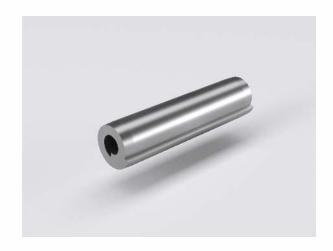
Coiled spring pins consist of 2 1/4 coils of spring steel or stainless steel and have swaged chamfers at each end. They are designed for plain drilled holes, but countersinking makes insertion easier.
